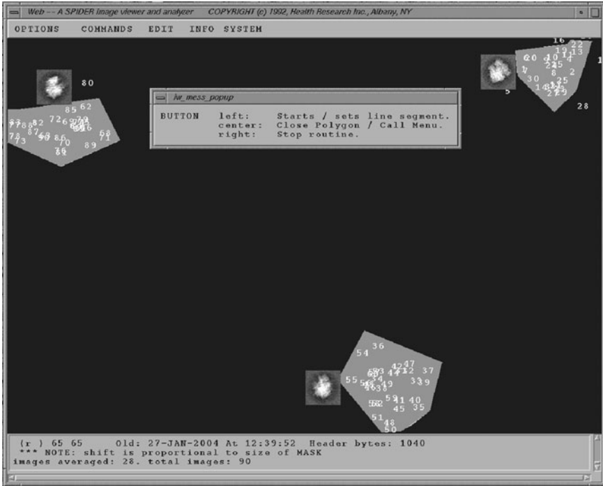
Figure 4.13 “Local” averages of ribosome images in factor space. An interactive tool (in this case, WEB; Frank et al., 1996) allows polygonal boundaries to be drawn in a factor map, to identify images to be averaged. Here, this action allows the three main views of the ribosome to be recovered (see the noise-free projections in the first column of figure 4.10).
